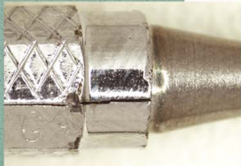
Figure 1. Crack in instrument handle.
